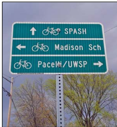
Figure 39: Wayfinding Signs Wayfinding signs indicate the direction and distance to specific destinations for bicyclists. Wayfinding signs can be used to enhance bicycle facilities including bike lanes, bike boulevards, and shared use paths. Signs can help bicyclists navigate the bicycle network and can be placed at key intersections to guide users to specific destinations. They can include the distance to those locations and approximate travel time as well.
