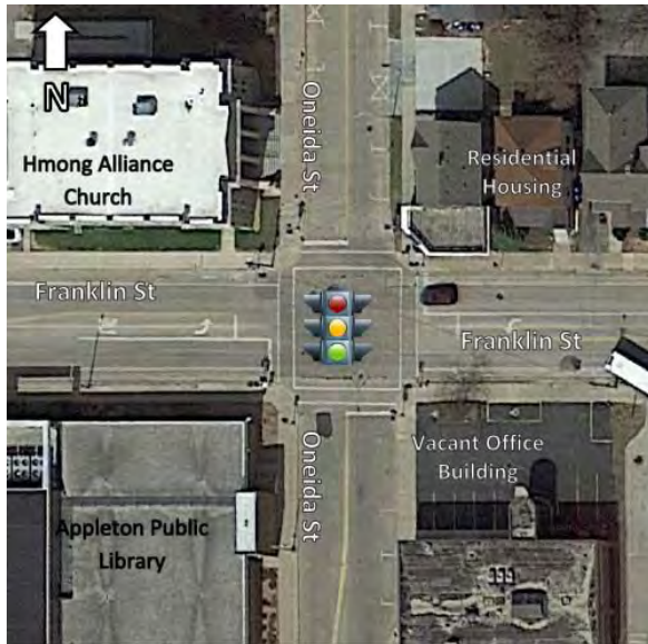
Figure 8: Franklin Street and Oneida Street Intersection The existing traffic signal at the Franklin Street and Oneida Street intersection is not warranted.
