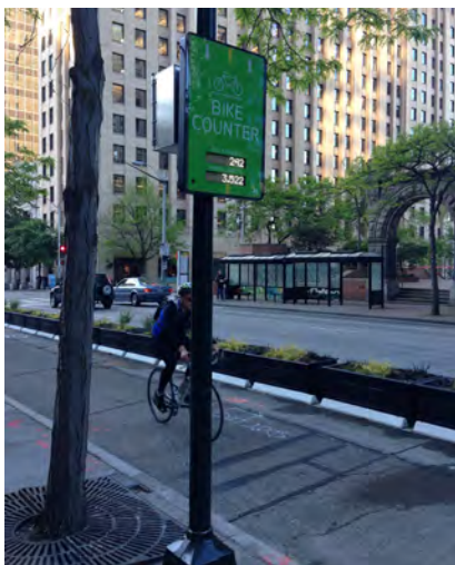
A bike counter on the Second Avenue cycle track in Seattle, WA provides real-time display of the number of bicyclists per day and year-to-date.
