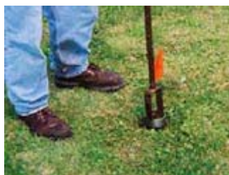
Field soil testing using hand auger.
