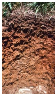
Depiction of healthy corn root structure and photo of silty clay loam soil profile to 30-inch depth.
